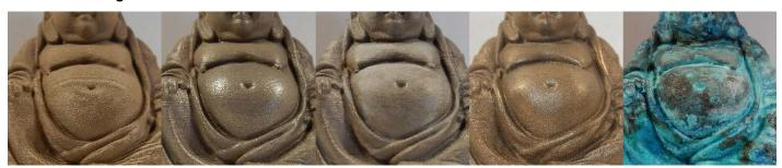
Post-processing the M-Fil range is quite an easy process though manual labour is required when you do not have access to an so called "rock tumbler" which gives the best polished results.
